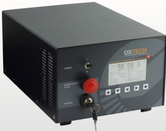
The product series ds11-t127 of table top drivers has all features of the ds-series. It is powered by an input voltage of 98~230VAC with power factor correction. The power ranges from 300W to 1200W. The laser diode current ranges up to 120A and voltage up to 48V.
