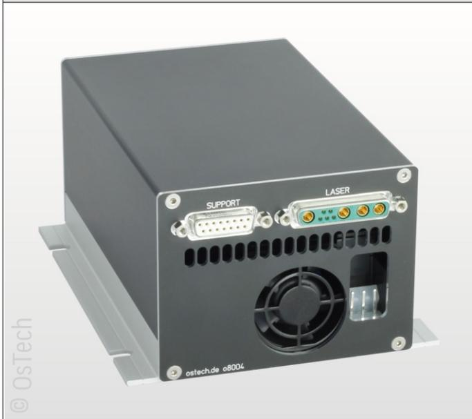
The product series ds11-o80 of OEM drivers has all features of the ds-series. It is powered by an input voltage of 110~230VAC with power factor correction. The power ranges from 150W to 600W. The laser diode current ranges up to 80A and voltage up to 48V.
