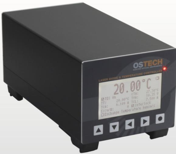
The product series ps11-t85 of table top drivers has all features of the ds-series. It is powered by an input voltage of 98~230VAC with power factor correction. The power ranges up to 460W. The TEC current ranges up to 20A and voltage up to 48V.
