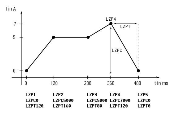
The commands for defining this sequence are shown below the corresponding points. For example, point 4 is selected with LZP4. Then the current target of 7 A is entered by LZPC7000. The command LZPT120 sets the time until the next point to 120 ms. This sequence ends after reaching point 5, because the time of point 5 is set to 0.
